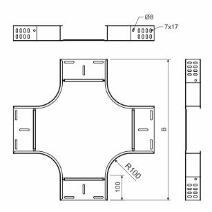
product description: The cross-over is used to connect cable trays that cross over on one level running through JUPITER cable trays or cable
